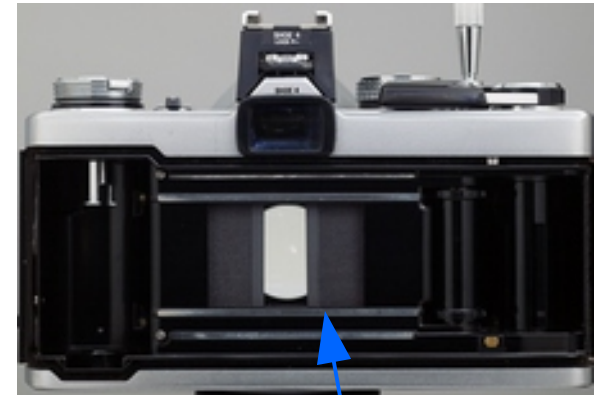
shutter: mechanical or electronic mechanism to limit light collection to a specific time period
