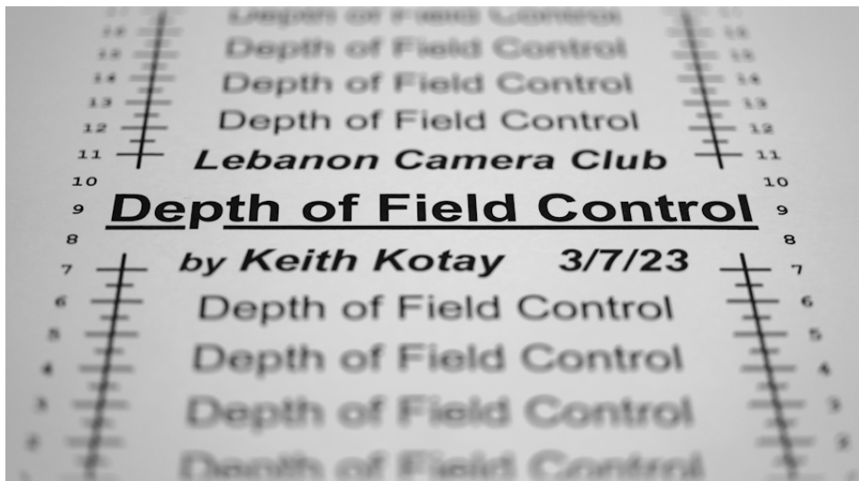
shallow depth of field (paper at a 45° angle, bottom closest to camera)
