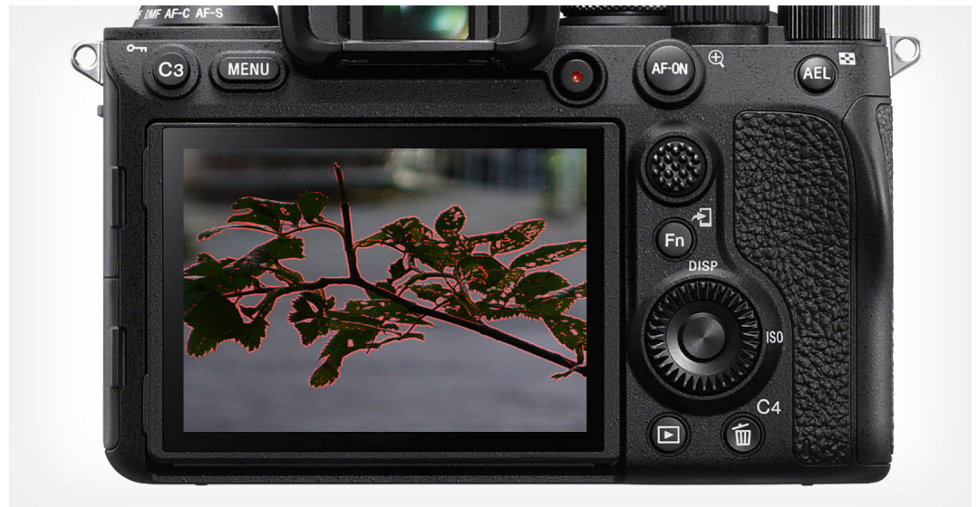
focus peaking highlights high contrast edges to show the area in focus
