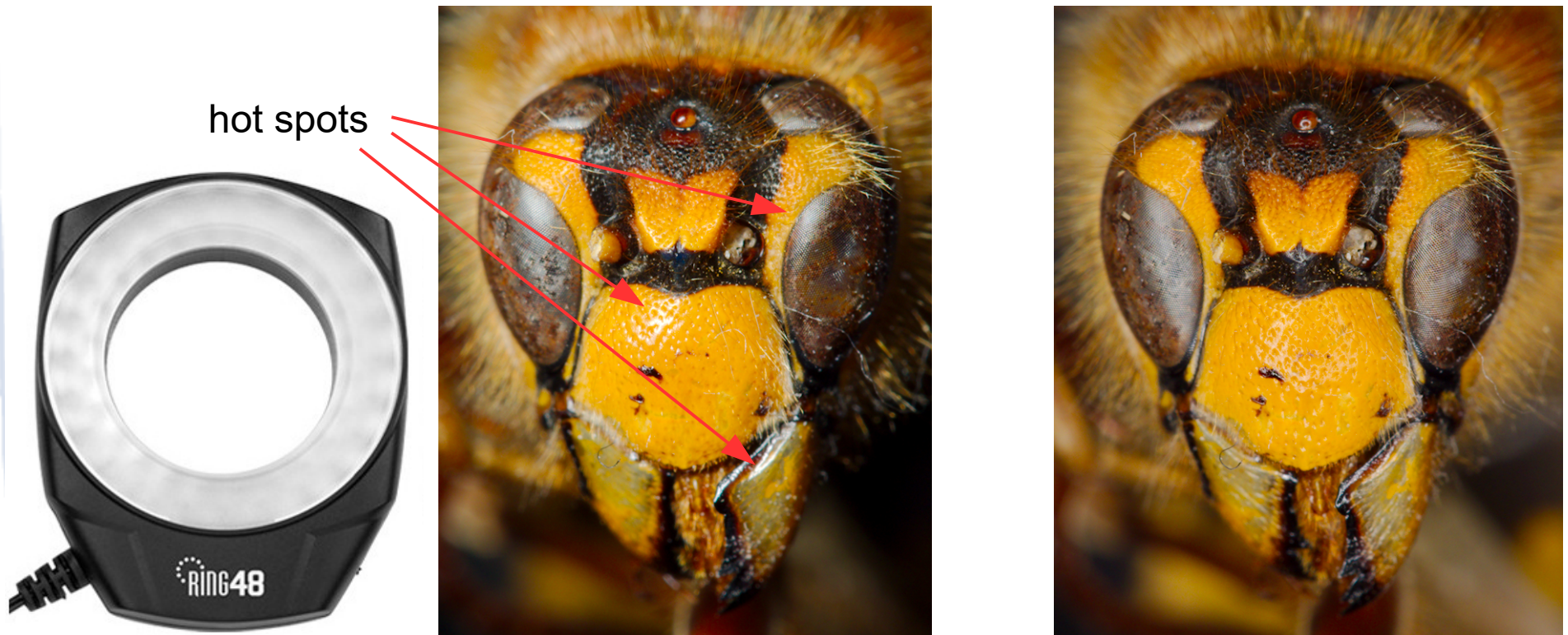
normal light, left → uneven illumination ring light → even illumination
